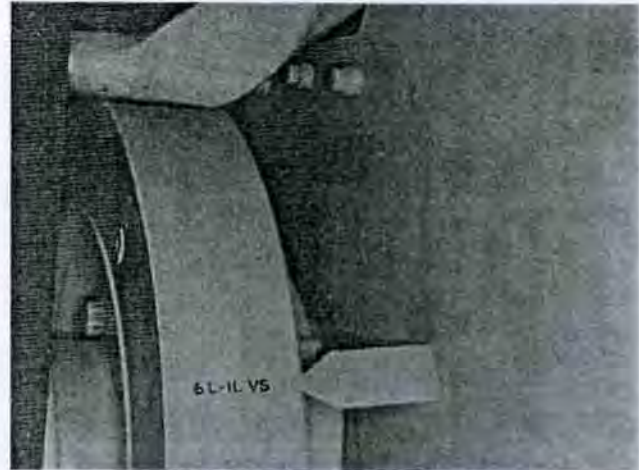
Fig. 2-59, (K21917). Valve set marks on vibration damper — KT/KTA38
